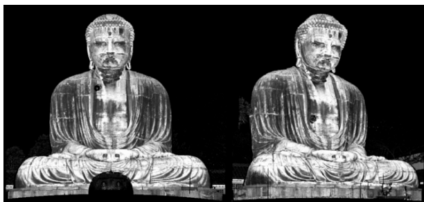
Figure 5.2. Images using laser reflectance strength as pixel values.
