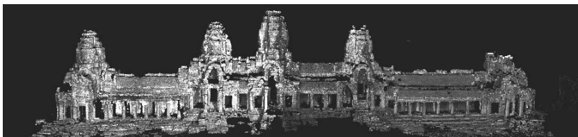
Figure 14.1. The texture of the Bayon Temple in Angkor, Cambodia. The color of the objects varies due to the use of textures taken at different times.
